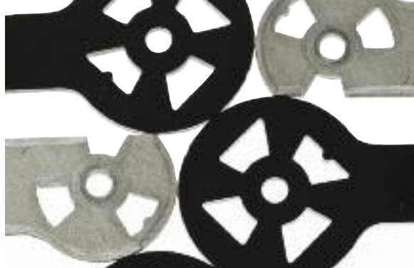
A change in tool coatings at Cowles Stamping increased punch life from 3000 to 16,000 hits between sharpenings when stamping HSLA-steel automotive parts.
