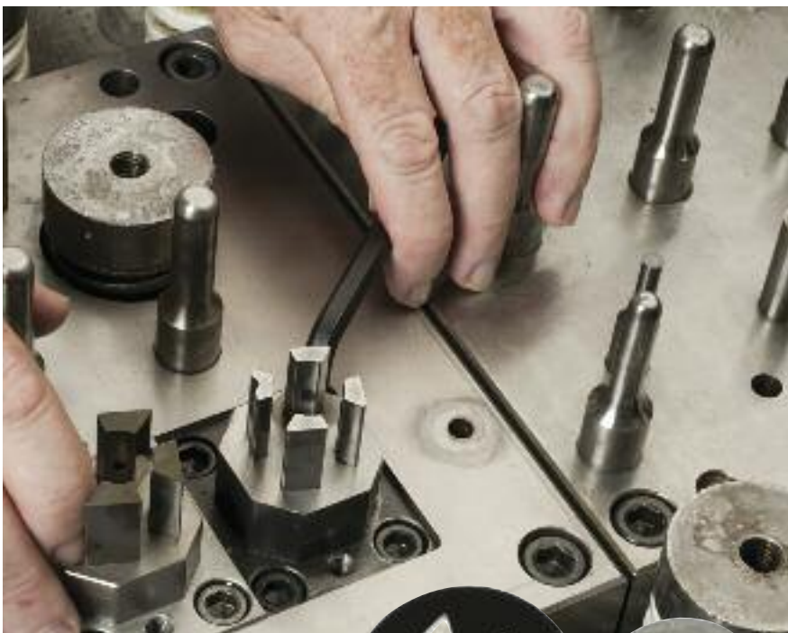
A change in tool coatings at Cowles Stamping increased punch life from 3000 to 16,000 hits between sharpenings when stamping HSLA-steel automotive parts.
