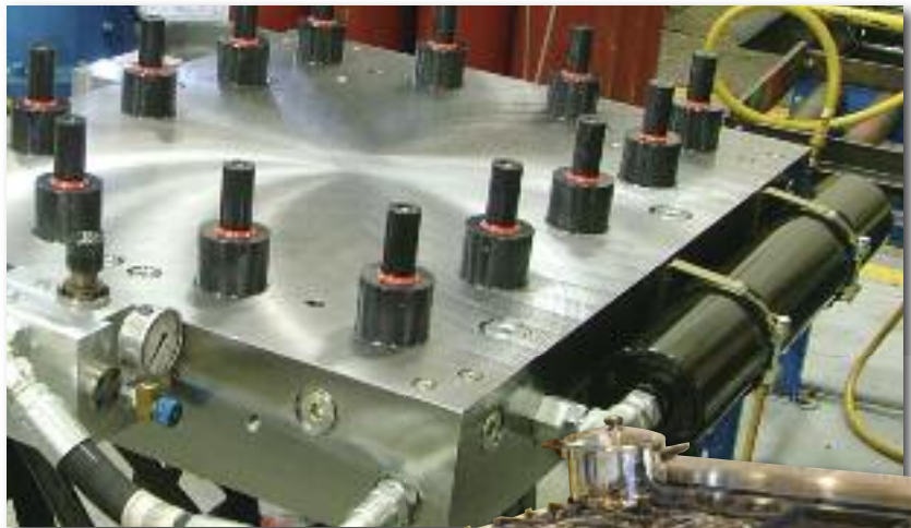
Adding a programmable hydraulic cushion to this die, which stamps a stainless-steel range top, eliminated the need to use a press equipped with a programmable cushion.
