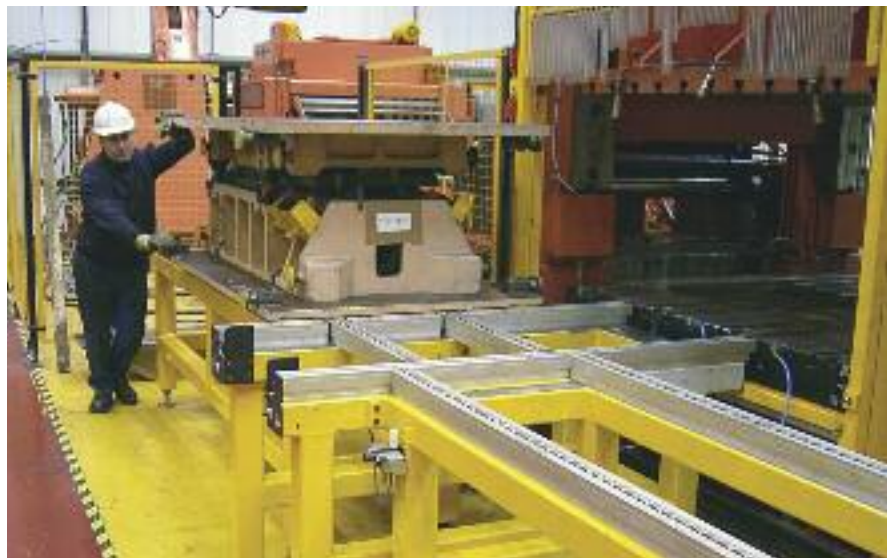
Using a dedicated die-change table will avoid die-change delays caused by waiting for a multitasking fork truck or overhead crane to become available.
