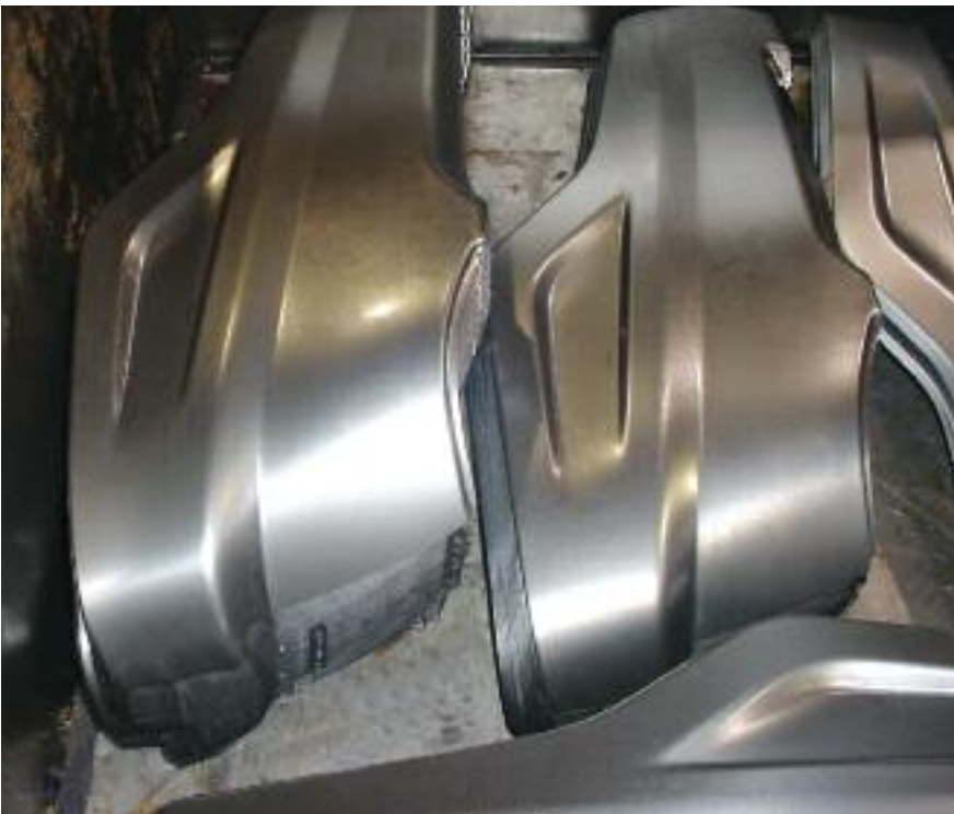
Deep drawing these mower decks at line speeds to 12 strokes/min. can generate a lot of heat. Any lubrication failings can quickly lead to galling and other premature die-wear issues caused by overheating.
