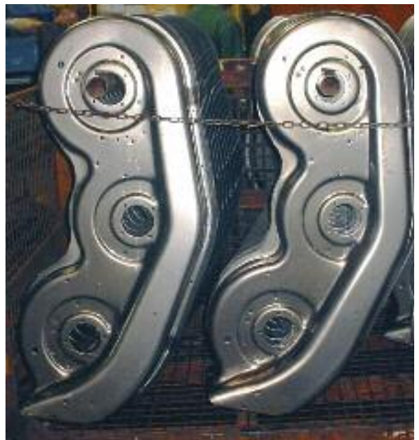
Deep-drawn mower side panels formed through a four-press cycle using multiple tools, ready to be washed and painted.
