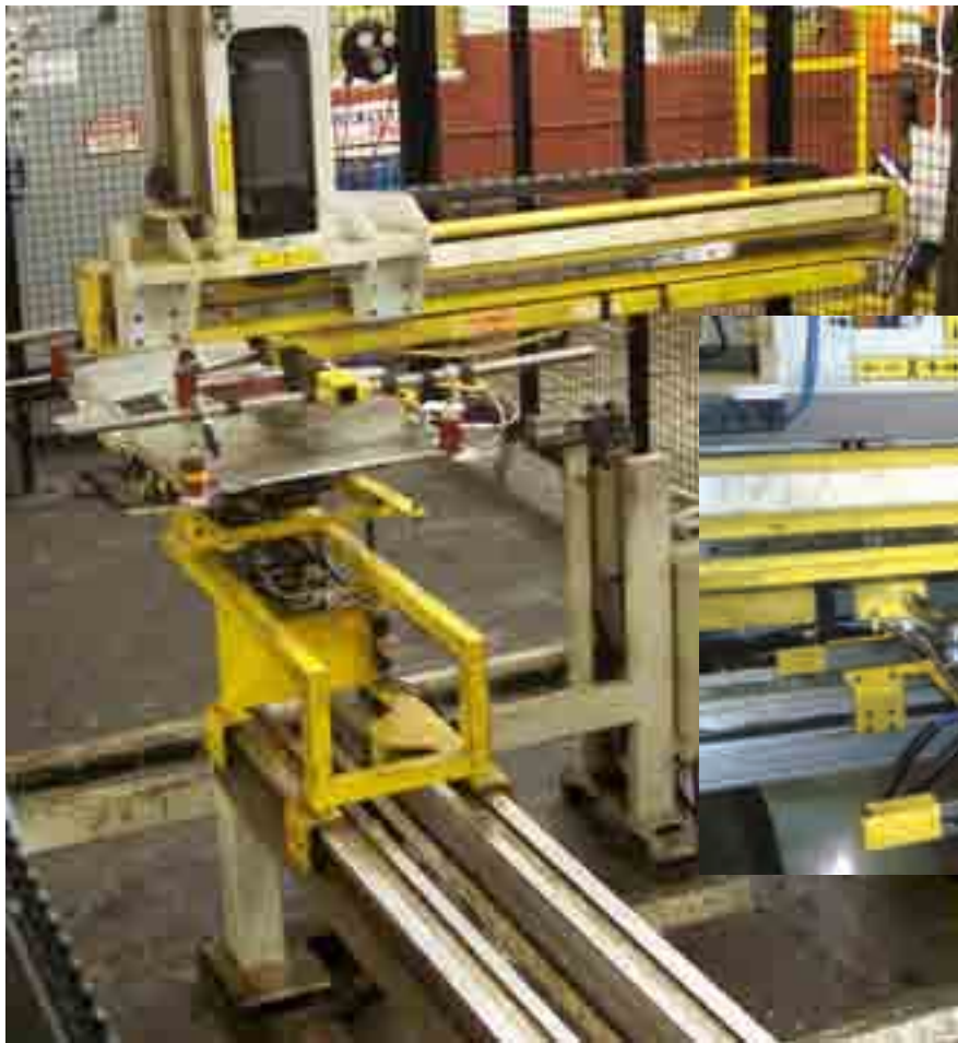
Press-tending press-mounted robots (below) on the roof-reinforcement line move blanks in and out of presses as servo-actuated shuttles (left) convey stampings between presses.
