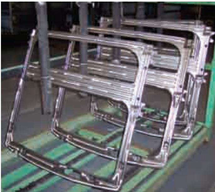
These stamped roof-reinforcement assemblies resistance-weld to prepared roof panels.
