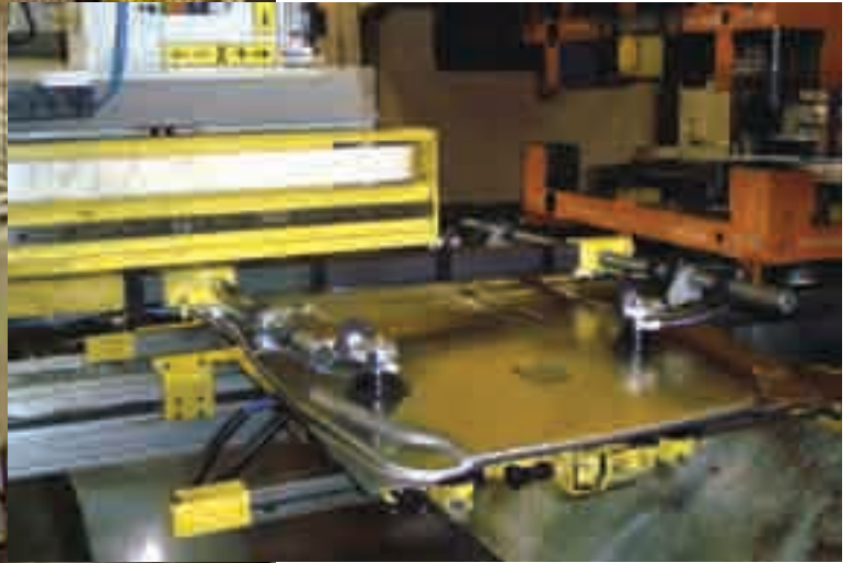
Press-tending press-mounted robots (below) on the roof-reinforcement line move blanks in and out of presses as servo-actuated shuttles (left) convey stampings between presses.
