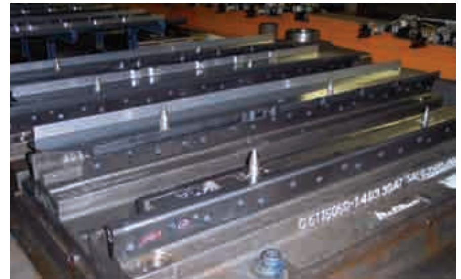
The sill-inner production die holds 16 of these rotary forming tools (from Ready Technology), which measure 29 in. long with 2-in.-dia. rockers. It takes two tools per 59-in. bend for a total of four tools per part. The tools transfer press vertical motion into a rotary forming operation, allowing overbending past 90 deg. while dramatically reducing required press tonnage.
