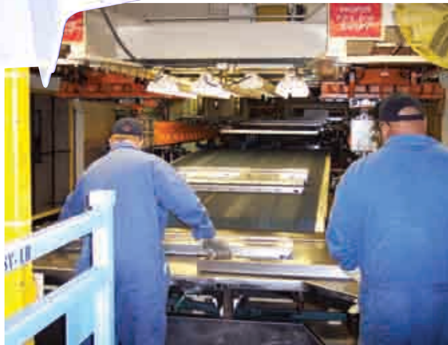
The sill-inner stampings, which measure 59.5 in. long, exit the 120-in. Verson transfer press four-out. After wiping the flanges upward, the die's rotary-bending tools form the channel. Notice the nicely even and straight impact lines at the channel bends, one thing the Daimler-Chrysler operators look for as they visually inspect the parts exiting the press.
