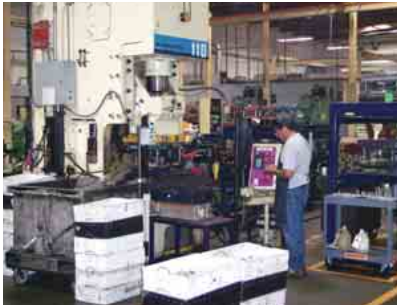
As part of its lean-manufacturing initiative, Walker Corp. has arranged many of its presses in workcells, surrounded by press-specific tooling. Such setups allow for rapid JIT production and promote improved productivity.
