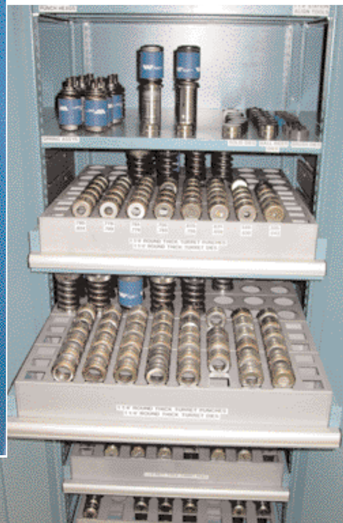
Managers and operators must agree on a standard location for every tool not in use, so that the tools required for a job can be easily found. Ways to achieve this include creating a shadow board (above) that indicates a place for storing every tool, and maintaining well-organized die cabinets (right).
