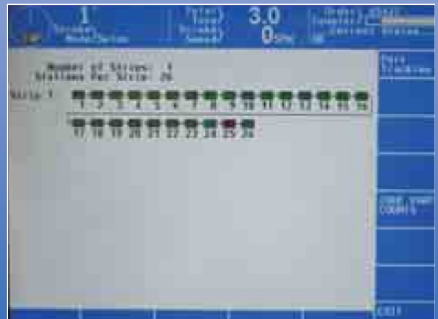
Now the bad part resides in the ejection station of tool 25. During this stroke, the PLS activates to move the part diverter into place so that the part ejects into a scrap bin.
