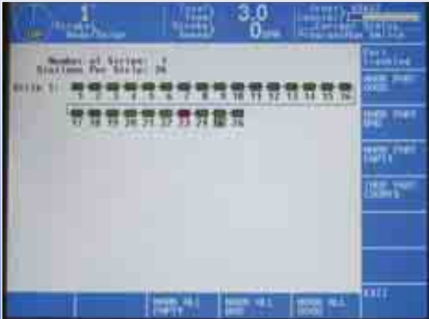
The control's shift register displays station 23 in red to indicate a bad part due to a missing insert.
