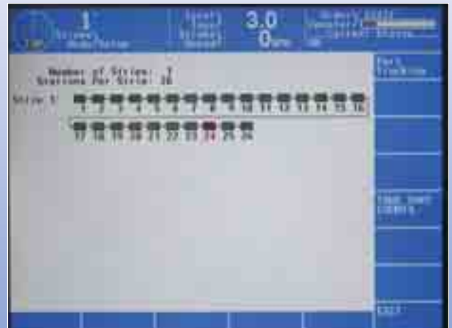
The screen indicates the bad part moving through the tool—here it's shown at station 24.
