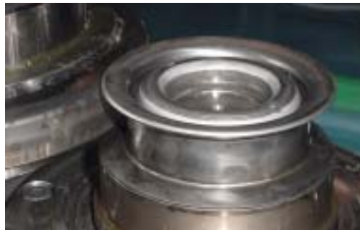
The Gill one-piece spinformed idler pulley, shown in the tooling after forming.
